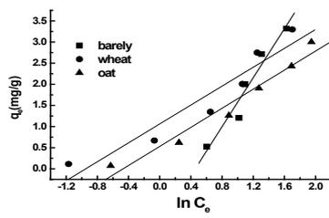
Figure 5. Temkin isotherm plots for the adsorption of MB by unsoaked straws (temperature = 30 °C, contact time =180 min)
