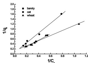
Figure 1. Langmuir isotherm plots for adsorption of MB by unsoaked straws (temperature= 30°C, contact time =180 min)
